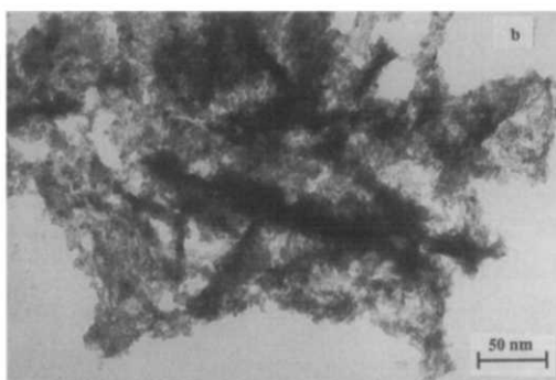
Fig. 12. TEM images of typical cerium oxides prepared in 25 \text{ mol kg}^{-1} NaOH: (a) with hexahydrated cerium(III) nitrate precursor, and (b) with tetrahydrated cerium(IV) sulphate precursor.
